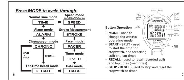
This is only a brief description of these buttons. Detailed uses of the buttons are different in particular functions and will be described later in the instructions.
